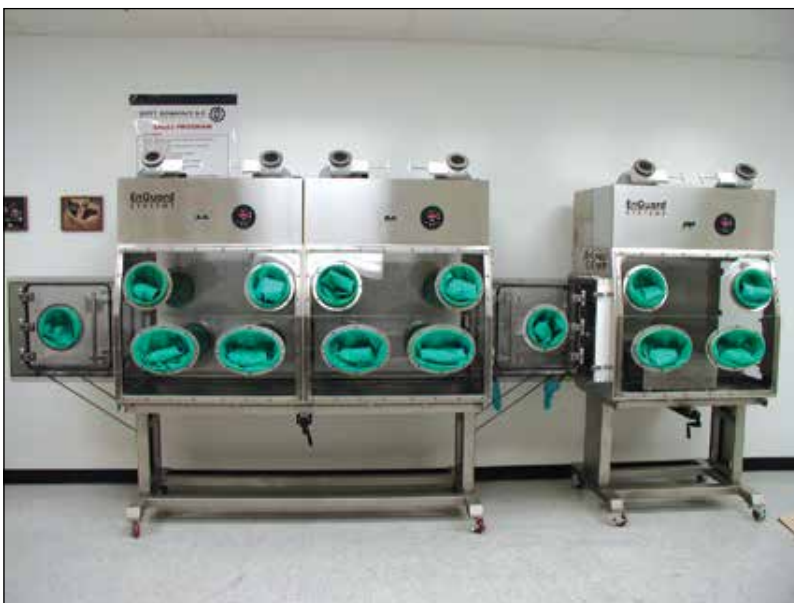
Manual Filling and Weighing Isolation System.
